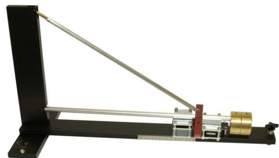
Fig 2. The SEP Seismometer in use in the School Seismology Project
